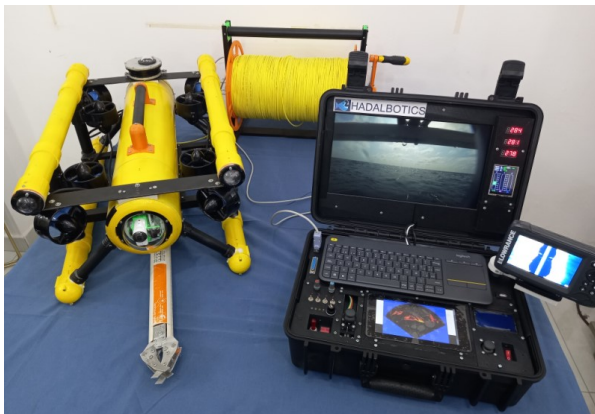
Fig. 2 HAUV Prototype rated for 1000 m of depth working as ROV: underwater vehicle, tether and surface control station.
